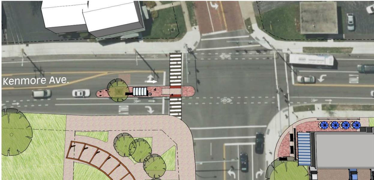
Figure 10: By eliminating the left hand only turn lane, space is created within the street cross-section to accommodate an in-street boarding island bus stop. This will enable transit users to cross the right hand only turn lane and bike lane when it is safe to do so, and wait for the bus at the in-street boarding island.
