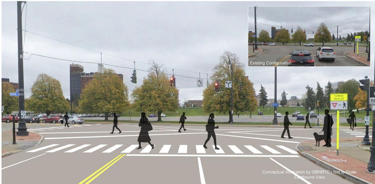
Figure 8: Illustration of the pedestrian scramble concept at the intersection of Main Street, Kenmore Avenue and the new South Campus entrance, looking towards the campus (illustration by GBNRTC)
