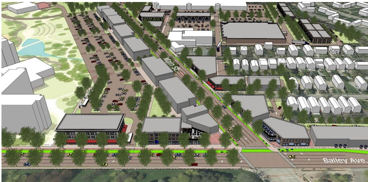
Figure 3: Birds-eye view of the intersection of Main Street and Bailey Avenue showing the proposed protected cycle tracks
