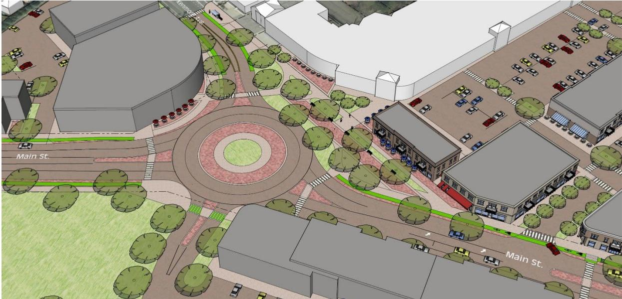
*Figure 6: Birds-eye view of Option 1 for the intersection of Main Street, Kenmore Avenue and the new South Campus entrance alternative with roundabout (requires further study)*
