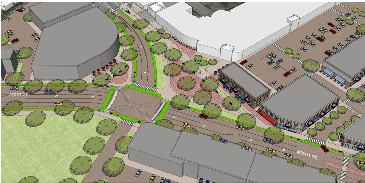
*Figure 7: Birds-eye view of Option 2 for the intersection of Main Street, Kenmore Avenue and the new South Campus entrance alternative with enhanced pedestrian/bike crossings and traffic signals with pedestrian scramble phase*
