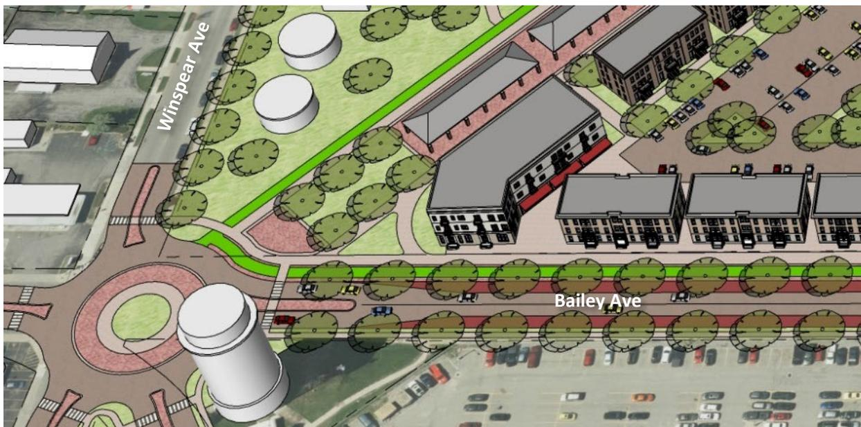
Figure 9: The roundabout proposed at the intersection of Bailey Avenue, Winspear Avenue and LeBrun Road would improve traffic flow and anchor the terminus of a pedestrian spine with community gathering space connecting the intersection to South Campus. The two-way separated cycle track proposed for the west side of Bailey Avenue and the proposed bus rapid transit lanes on Bailey Avenue are also illustrated.
